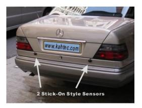
Blinking Smart Eye is available with 2, 3, or 4 sensors in either the standard Drill-Hole type style or the special Stick-On type style.
